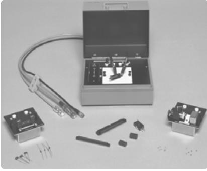
**Agilent 16339A component test fixture**
