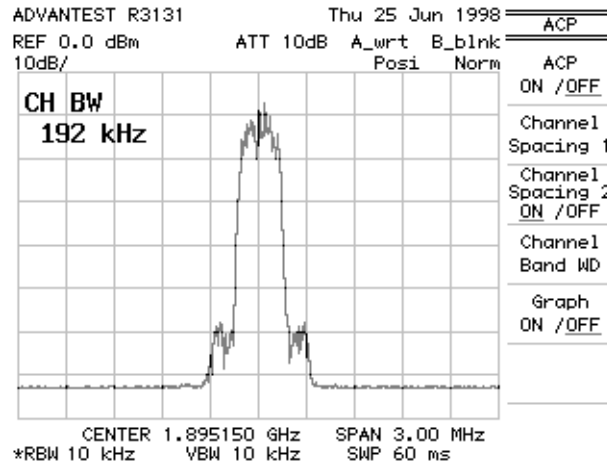
Figure 2-64 Setting the Specified Bandwidth
